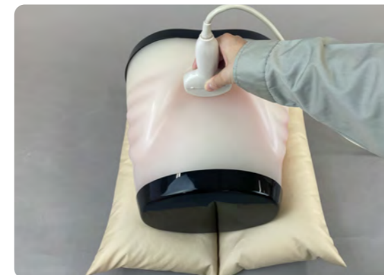
1. The phantom can be scanned with actual ultrasound devices. * The map of simulated targets is on the backside of this manual.
