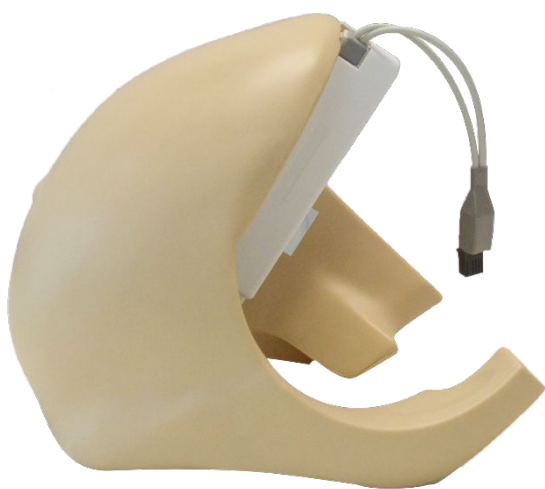
a. Abdominal unit This unit is attached to the abdomen of the maternal models (Hana and the Delivery Assistance Model).
