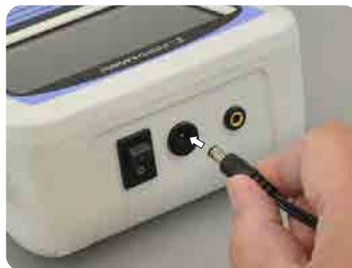
3. Connect the AC adapter to a power source and turn on the power.
