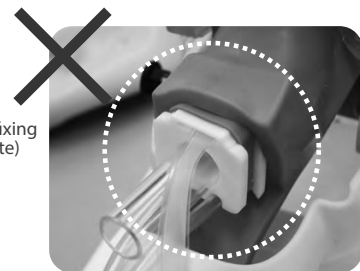
Example of inappropriate installation of tongue component
