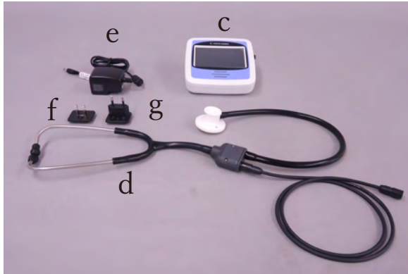
c. controller d. simulated stethoscope e. AC adapter f. slide plug attachment type A g. slide plug attachment type C
