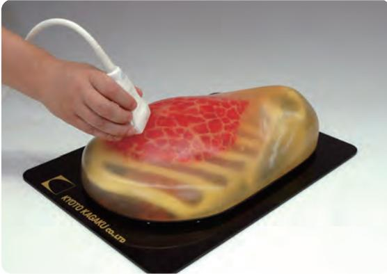
① The phantom can be scanned with real ultrasound devices.
