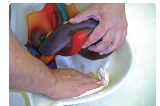
② Wipe the container walls and the phantom by soft cloth and make them dry before storage.
