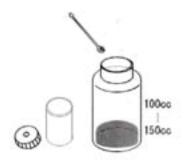
A-1. Put a little pinch of the coloring powder and 100-150cc of the water into the injection bottle and stir together.
