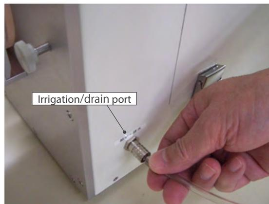
Connect the water-filled syringe to the tube from the irrigation/drain port (lower port). Fill the water until you see water flow out from the vent port.
