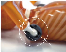
Shoulders: rotate full 360 degrees in the sagittal plane, approx. 180 degrees to side-ways.
